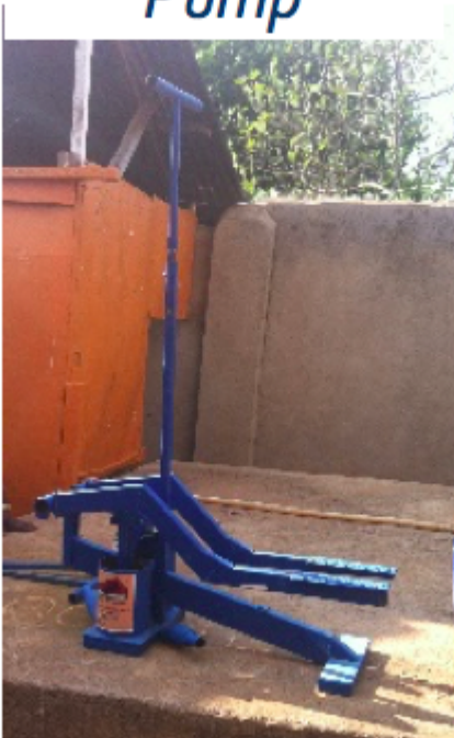
Fig. 2: Treadle pump to access water from tank
